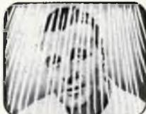
**STREBS**—Caused by car ignition, trucks or buses or by Neon signs, door bells, electric toasters, broilers, radios and phonographs. TELERON WAVE TRAP eliminates this interference BEFORE IT REACHES YOUR SET.
